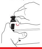
To attach Red Plus Palm Support, line up both units as shown. The tongue that runs along Red Plus Palm Support fits inside the groove that runs along front edge of RollerMouse Red, between the two red end caps.
